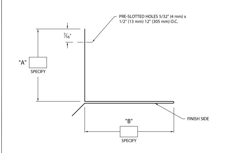
NOTE: 3 1/2" (89 mm) CONCEALED SPLICE PLATE PROVIDED AT EACH JOINT.
