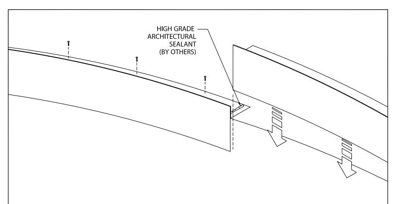
STEP 1 - POSITION AND FASTEN 4'-0" GRAVEL STOP SECTION 6" O.C. AS SHOWN WITH PROVIDED NAILS. LEAVE 3/8" GAP BETWEEN SECTIONS
