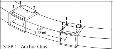
Locate and fasten 8" wide anchor clips at 4'-0" (1.22 m) O.C. with provided fasteners for substrate (see detail A).
