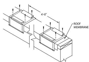
STEP 7 - ANCHOR CLIPS LOCATE AND FASTEN GALVANIZED ANCHOR CLIPS TO WALL AT 4'-0" CENTERS WITH PROVIDED FASTENERS FOR SUBSTRATE USING THE THIRD FULL TOP HOLE FROM THE BEND (SEE DETAIL A)
