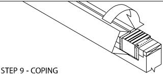
HOOK OUTSIDE FACE OF COPING OVER THE ANCHOR CLIPS AND ROTATE INTO PLACE. ENGAGE REAR LEG ONTO ANCHOR CLIPS BY PRESSING DOWNWARD UNTIL SNAP LOCK OCCURS.
