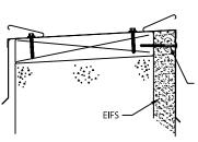
If using an EIFS system, fasten through face w/ fastener of proper length to penetrate nailer
