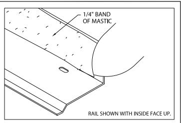
2. Miter & Scupper Base Rail (Preparation) Lay miters and spillout scuppers on deck with outside face down. Be sure aluminum base rail is clean and free of dirt or dust. Apply a heavy 1/4" band of approved mastic/sealant to the back of the deck flange to entire length of base rail as shown. Application of sealant is required along the full length of each miter base rail.
