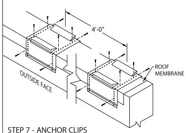
LOCATE OVER ROOFING MEMBRANE
