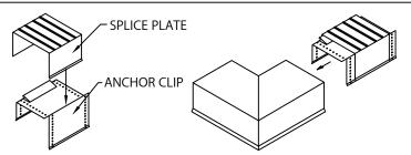
STEP 2 - MITER SPLICE PLATES & ANCHOR CLIPS REMOVE RELEASE PAPER FROM SPLICE PLATE SEALANT STRIPS. POSITION THE SPLICE PLATE IN THE CENTER OF THE ANCHOR CLIP. INSTALL THE SPLICE PLATE AND ANCHOR CLIP ASSEMBLIES HALFWAY INTO EACH END OF THE CORNER MITER AS SHOWN.
