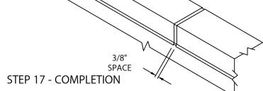
USING STRAIGHT LENGTH SECTIONS TO COVER ALL EXPOSED CLIPS / SPLICES, CUT TO LENGTH AS NEEDED USING A FINE TOOTH HACKSAW, SNIIPS, OR CUT-OFF WHEEL LEAVING A CLEAN EDGE. BE SURE TO LEAVE A 3/8" SPACE AT EACH JOINT.
