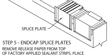
OF FACTORY APPLIED SEALANT STRIPS. PLACE
