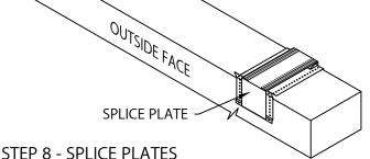
PLACE SPLICE PLATE ONTO ANCHOR CLIPS AT SPLICE JOINTS, 12'-0" O.C. NOTE: REMOVE RELEASE PAPER FROM SEALANT STRIPS.
