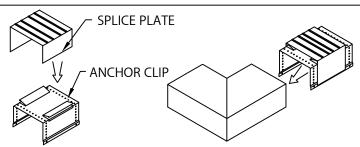
STEP 2 - MITER SPLICE PLATES & ANCHOR CLIPS POSITION THE SPLICE PLATE IN THE CENTER OF THE ANCHOR CLIP. INSTALL THE SPLICE PLATE AND ANCHOR CLIP ASSEMBLY INTO EACH END OF THE CORNER AS SHOWN
