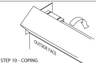
HOOK OUTSIDE FACE OF COPING OVER THE ANCHOR CLIP/ENDWALL FLASHING AND ROTATE INTO PLACE. ENGAGE REAR LEG ONTO ANCHOR CLIP BY PRESSING DOWNWARD UNTIL SNAP LOCK OCCURS. NOTE: REMOVE PLASTIC PROTECTIVE FILM IMMEDIATELY.
