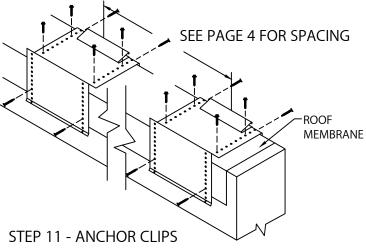
LOCATE AND FASTEN GALVANIZED ANCHOR CLIPS TO WALL AT CENTERS WITH PROVIDED FASTENERS FOR SUBSTRATE SEE COPING ANCHOR CLIPS AND SPACING ON PAGE 4.
