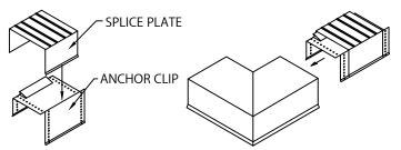
STEP 2 - MITER SPLICE PLATES & ANCHOR CLIPS REMOVE RELEASE PAPER FROM SPLICE PLATE SEALANT STRIPS. POSITION THE SPLICE PLATE IN THE CENTER OF THE ANCHOR CLIP. INSTALL THE SPLICE PLATE AND ANCHOR CLIP ASSEMBLIES HALFWAY INTO EACH END OF THE CORNER MITER AS SHOWN.
