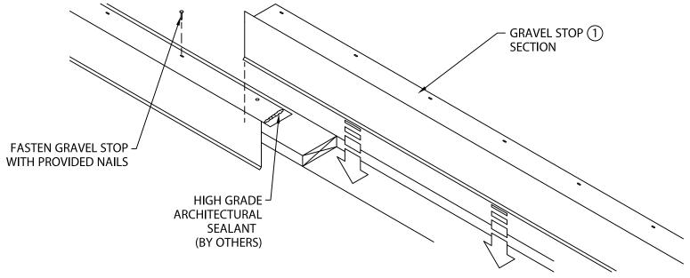
STEP 1 POSITION GRAVEL STOP AND FASTEN EACH SECTION THROUGH HOLES PROVIDED 6" O.C. WITH PROVIDED NAILS. SEALANT (BY OTHERS) TO BE FIELD APPLIED AS SHOWN.
