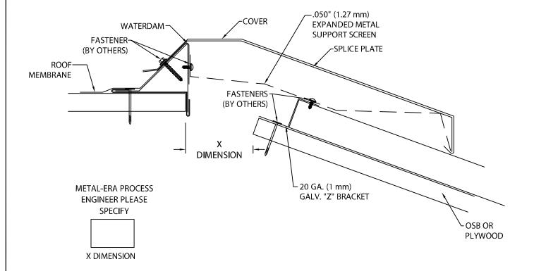
CAUTION! INSTALLERS SHALL WEAR PROTECTIVE EYE WEAR TO PREVENT INJURY. DO NOT OVERDRIVE FASTENERS, AS STRIPPING CAN OCCUR AT HIGH DRIVER TORQUE. RECOMMENDED DRIVING TOOL: 600 - 800 rpm ELECTRIC DRILL EQUIPPED WITH DEPTH-SENSING NOSE-PIECE TO PREVENT DRIVING AND STRIPOUT. DO NOT USE IMPACT TYPE TOOL.
