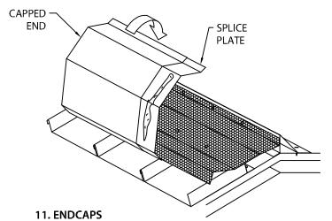
HOOK COVER DRIP ONTO EXPANDED METAL SUPPORT SCREEN AND ROTATE INTO PLACE.
