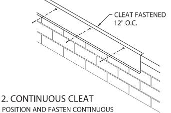
POSITION AND FASTEN CONTINUOUS CLEAT 12" O.C. THRU PRE-SLOTTED HOLES AS SHOWN WITH PROVIDED NAILS. LAP CLEAT 1" AT JOINTS.
