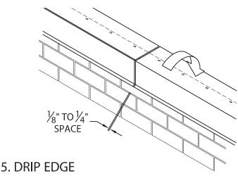
CONTINUE INSTALLING LENGTHS OF DRIP EDGE. LEAVE A  $\frac{1}{8}$ " TO  $\frac{1}{4}$ " SPACE BETWEEN PIECES.
