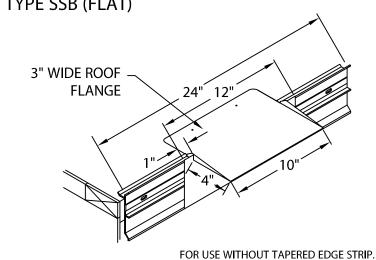
FLANGE FLUSH MOUNTED WITH ROOF.
