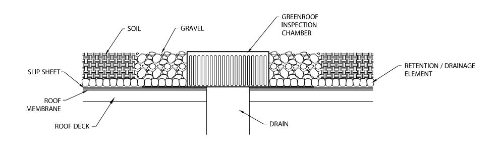
THE INSPECTION CHAMBER MAY BE INSTALLED DIRECTLY ON THE RETENTION / DRAINAGE ELEMENT IN THE GARDEN ROOF ASSEMBLY OR DIRECTLY OVER THE ROOT BARRIER PROTECTION FOR THE MEMBRANE.
