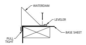
WATERDAM MUST BE PULLED TIGHT TO THE OUTSIDE FACE OF THE BUILDING BEFORE NAILING THE ROOF FLANGE.
