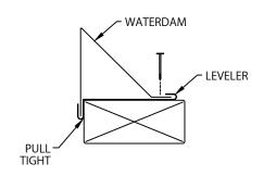
WATERDAM MUST BE PULLED TIGHT TO THE OUTSIDE FACE OF THE BUILDING BEFORE NAILING THE ROOF FLANGE.
