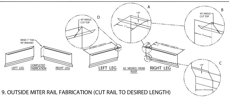
RIGHT LEG - DETAIL A: First remove a 1" section from top flange, 1/8" down face and 1" horizontally as shown to create tab. DETAIL B: Cut top flange at 45° angle. DETAIL C: Cut off bottom face at a 1/8" x 1" as shown and continue through area shown on bottom flange. Bend tab inwards 90°. LEFT LEG - DETAIL D: Trim top flange at a 45° angle.
