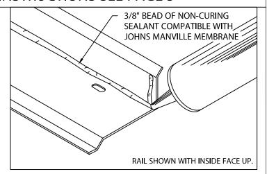
2. Miter & Scupper Base Rail (Preparation) Lay miters and spillout scuppers on deck with outside face down. Be sure aluminum base rail is clean and free of dirt or dust. Apply a heavy 3/8" bead of non-curing sealant to the right angle intersection of the deck flange and back of base rail as shown. Application of mastic is required along the full length of each miter base rail. Apply a similar 3/8" bead of sealant to the flange's left end, as you look at the outside face of the rail section.
