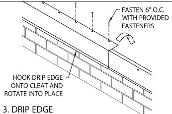
HOOK DRIP EDGE OF EACH DRIP EDGE SECTION ONTO CONTINUOUS CLEAT, ROTATE INTO PLACE. FASTEN THRU PRE-SLOTTED HOLES 6" WITH PROVIDED FASTENERS.
