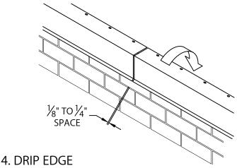
PROVIDED FASTENERS. LAP CLEAT 1" AT JOINTS.
