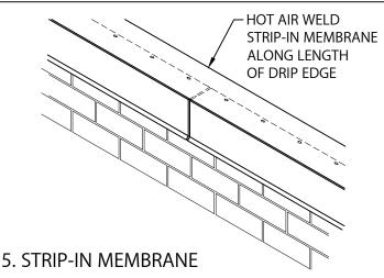
HOT AIR WELD STRIP-IN MEMBRANE ALONG ENTIRE LENGTH OF DRIP EDGE PER MANUFACTURERS INSTRUCTIONS.
