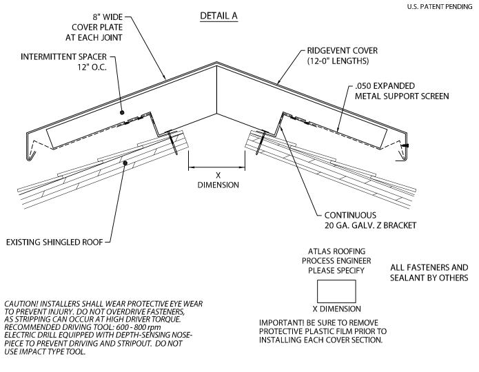
NOTE: ALL FASTENERS MUST MEET MINIMUM 240 LB. PULL-OUT FOR SUBSTRATE.
