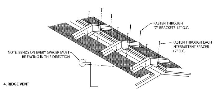
SET RIDGE VENT IN PLACE CENTERED OVER RIDGE OPENING. THE BENDS ON TOP OF THE SPACER MUST ALL BE FACING AWAY FROM THE END OF THE ROOF. FASTEN THROUGH PRE-PUNCHED SLOTTED HOLES IN INTERMITTENT SPACERS AT 12" O.C. WITH APPROPRIATE FASTENERS. ALSO FASTEN THROUGH PRE-PUNCHED SLOTTED HOLES IN "Z" BRACKETS 12" O.C.. LAP "Z" BRACKETS 1" ("Z" BRACKETS WILL LAP AND EXPANDED METAL SUPPORT SCREEN WILL BUTT UP TOGETHER).
