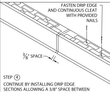
SECTIONS AS SHOWN. FIELD CUT AS NECESSARY.
