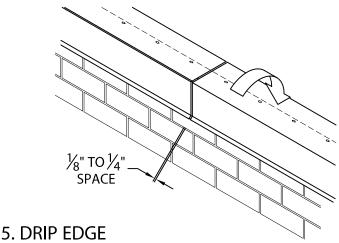
CONTINUE INSTALLING LENGTHS OF DRIP EDGE. LEAVE A  $\frac{1}{8}$ " TO  $\frac{1}{4}$ " SPACE BETWEEN PIECES.
