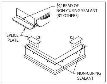
3. ANCHOR BAR MITER SPLICE PLATES APPLY A  $^3\!8$ " BEAD OF NON-CURING SEALANT (BY OTHERS) TO THE RIGHT ANGLE INTERSECTION OF THE DECK FLANGE AND TO EACH END OF ANCHOR BAR MITER. SLIDE 31/2" WIDE SPLICE PLATE HALFWAY ONTO EACH END OF MITER AS SHOWN.
