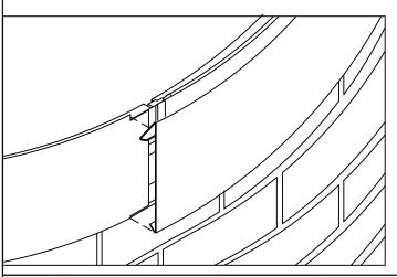
IMPORTANT! Anchor bar and fascia cover sections for radius walls are notched. Use care when removing from the box and when handling to avoid bending and kinking.
