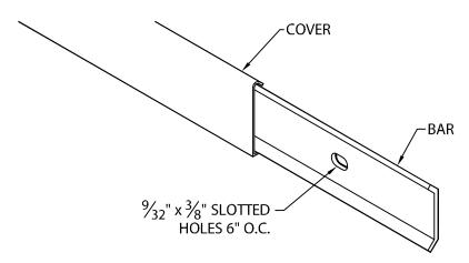
COVER PROVIDED WITH 1" LAP JOINTS SLOTTED FASTENING HOLES  $\%_{32}$ " x  $\frac{3}{8}$ " FURNISHED 6" O.C. NOTE: ALL MATERIAL .063" ALUMINUM UNLESS OTHERWISE NOTED
