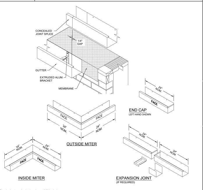
Standard gutter miter leg lengths are 24" Nominal Standard gutter miter angle is  $90^{\circ}\,$
