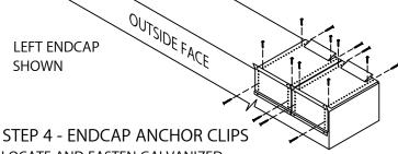
LOCATE AND FASTEN GALVANIZED ANCHOR CLIPS TO WALL WITH PROVIDED FASTENERS FOR SUBSTRATE (SEE DETAIL A).
