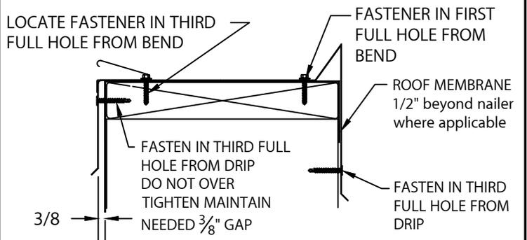
**ANCHOR CLIP FASTENING-DETAIL A**
