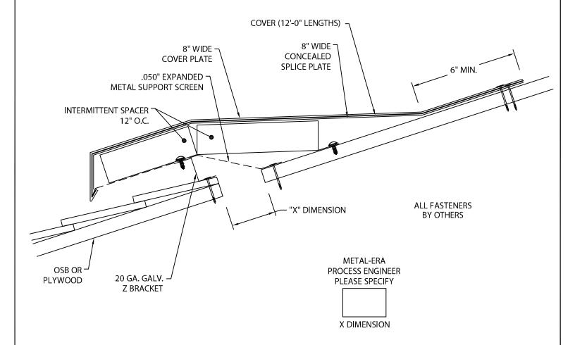
NOTE: ALL FASTENERS MUST MEET MINIMUM 240 LB. PULL-OUT FOR SUBSTRATE.
