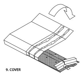
HOOK COVER INTO PLACE STARTING AT LOWER END. HOOK THE EXPANDED METAL SUPPORT SCREEN INTO THE COVER LIP. ROTATE COVER DOWNWARD.
