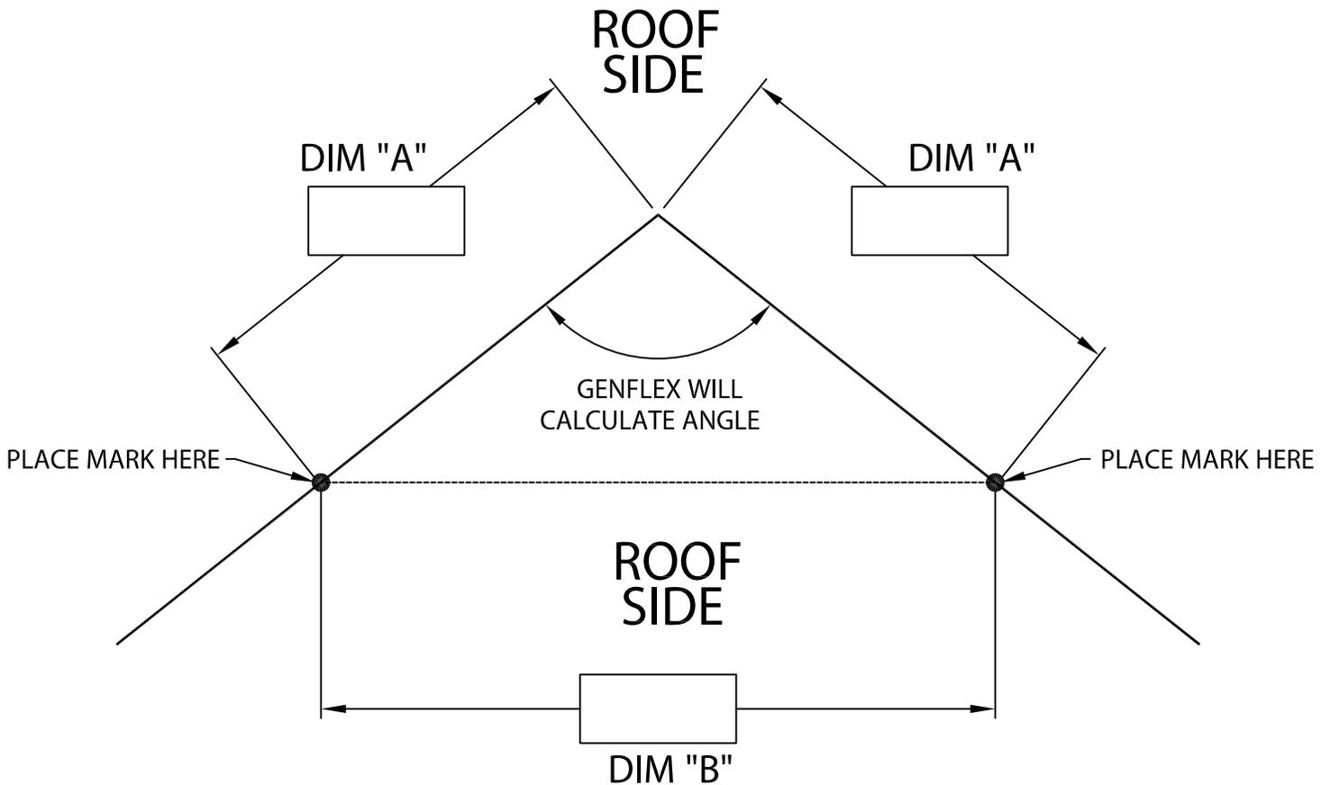
1. CIRCLE APPROPRIATE "ROOF SIDE" TO INDICATE OUTSIDE MITER OR INSIDE MITER. THIS DETAIL APPLIES FOR MITERS TIGHTER THEN 90° (ACUTE) OR WIDER THEN 90° (OBTUSE).
