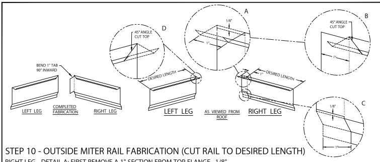
RIGHT LEG - DETAIL A: FIRST REMOVE A 1" SECTION FROM TOP FLANGE, 1/8" DOWN FACE AND 1" HORIZONTALLY AS SHOWN TO CREATE TAB. DETAIL B: CUT TOP FLANGE AT A 45° ANGLE. DETAIL C: CUT OFF BOTTOM FACE 1/8" x 1" AS SHOWN AND CONTINUE THROUGH AREA SHOWN ON BOTTOM FLANGE. BEND TAB INWARDS 90°. LEFT LEG - DETAIL D: TRIM TOP FLANGE AT A 45° ANGLE.
