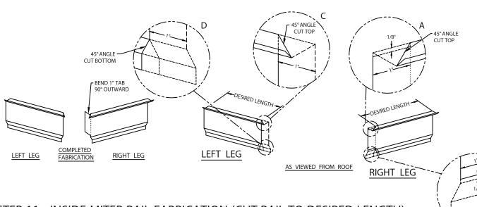
STEP 11 - INSIDE MITER RAIL FABRICATION (CUT RAIL TO DESIRED LENGTH)
