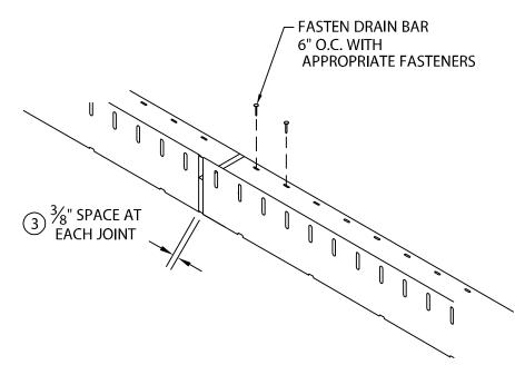
STEP 3 - CONTINUE BY INSTALLING DRAIN BAR SECTIONS ALLOWING A 3/8" SPACE BETWEEN SECTIONS AS SHOWN. FIELD CUT AS NECESSARY.
