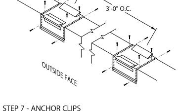
LOCATE AND FASTEN GALVANIZED ANCHOR CLIPS TO WALL AT 3'-0" CENTERS WITH PROVIDED FASTENERS FOR SUBSTRATE (SEE DETAIL A).
