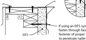
If using an EIFS system, fasten through face w/ fastener of proper length
