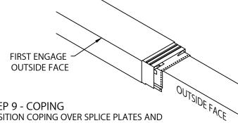
STEP 9 - COPING POSITION COPING OVER SPLICE PLATES AND PRESS DOWNWARD UNTIL OUTSIDE FACE CLEARS SPLICE PLATES. ENGAGE OUTSIDE FACE BY PUSHING DOWNWARD ON FRONT EDGE UNTIL SNAP LOCK OCCURS. THEN ENGAGE INSIDE FACE BY PUSHING DOWNWARD ON BACK EDGE UNTIL SNAP LOCK OCCURS.
