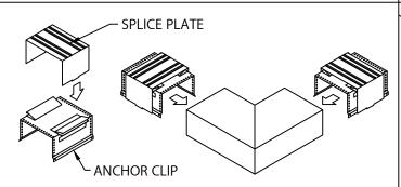
STEP 2 - MITER SPLICE PLATES & ANCHOR CLIPS POSITION THE SPLICE PLATE IN THE CENTER OF THE ANCHOR CLIP. INSTALL THE SPLICE PLATE AND ANCHOR CLIP ASSEMBLY HALFWAY INTO EACH END OF THE CORNER AS SHOWN.
