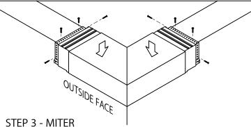
PLACE THE CORNER ASSEMBLY INTO POSITION AND SECURE AT THE EXPOSED EDGE OF THE ANCHOR CLIPS AS PER DETAIL A.
