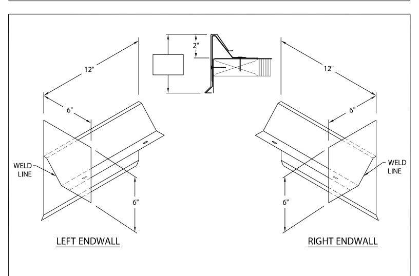
DIRECTION IS DETERMINED AS SEEN FROM ROOF SIDE
