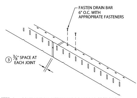
STEP 3 - CONTINUE BY INSTALLING DRAIN BAR SECTIONS
