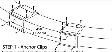
Locate and fasten 8" wide anchor clips at 4'-0" (1.22 m) O.C. with provided fasteners for substrate (see detail A).
