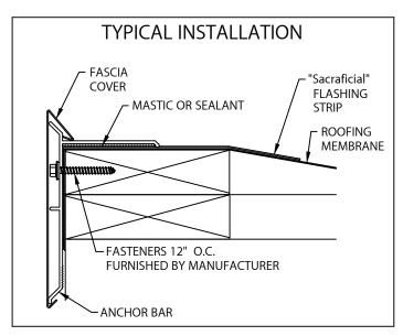
IMPORTANT! Be sure to remove protective film prior to installing each fascia section.
