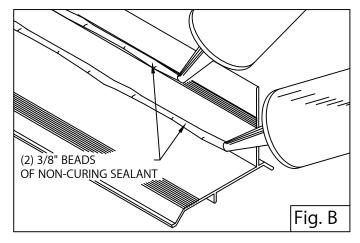
3. Miter & Scupper Anchor Bar (Preparation)
