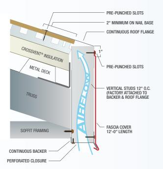
The above diagram shows the components of the Techni-Flo<sup> $\infty$ </sup> EV. Proper installation is required to achieve optimal airflow through the eave and to maintain warranty coverage. Go to www.AtlasRoofing.com for further installation instructions.
