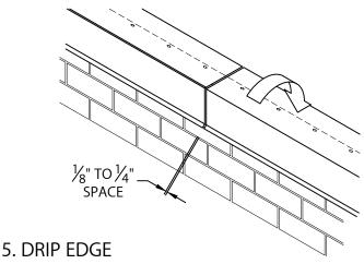
CONTINUE INSTALLING 10'-0" LENGTHS OF DRIP EDGE. LEAVE A  $\frac{1}{8}$ " TO  $\frac{1}{4}$ " SPACE BETWEEN PIECES.
