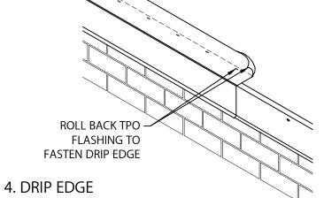
ROLL BACK TPO FLASHING TO EXPOSE FASTENING SLOTS AND FASTEN THRU PRE-SLOTTED HOLES 6" WITH PROVIDED FASTENERS.
