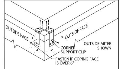
STEP 1 - CORNER SUPPORT CLIPS LOCATE AND FASTEN GALVANIZED CORNER SUPPORT CLIPS TO THE WALL. IF COPING FACE OVER 6", SECURE WITH ADDITIONAL FASTENER AS SHOWN.
