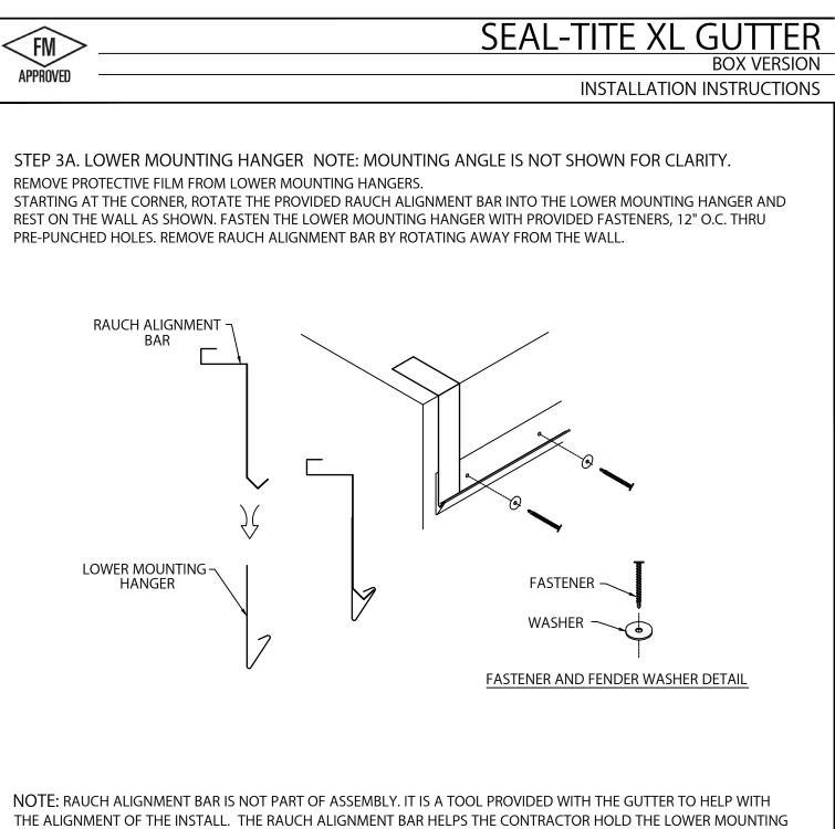
THE ALIGNMENT OF THE INSTALL. THE RAUCH ALIGNMENT BAR HELPS THE CONTRACTOR HOLD THE LOWER MOUNTING HANGER IN PLACE AS IT IS GETTING FASTENED TO THE WALL. THE RAUCH ALIGNMENT BAR IS INTENDED TO RECESS THE GUTTER TOP APPROXIMATELY  $\frac{1}{4}$ " FROM THE TOP OF THE WALL, TO ALLOW FOR WALL VARIATIONS.
