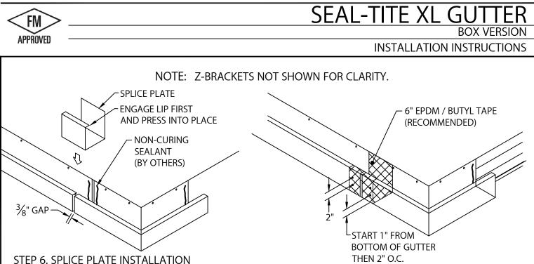
APPLY A HEAVY BEAD OF NON-CURING SEALANT TO INSIDE END OF GUTTER. LEAVE A 3/8" GAP AT SPLICE JOINT. PLACE 6" WIDE SPLICE PLATE AT JOINT. RIVET SECTIONS WITH PROVIDED  $\frac{1}{8}$ " STAINLESS STEEL POP RIVETS AT SPLICE JOINT 2" O.C. AS SHOWN, STARTING 1" FROM BOTTOM OF GUTTER. THE MANUFACTURER RECOMMENDS THE APPLICATION OF EPDM / BUTYL PRESSURE SENSITIVE TAPE CENTERED OVER THE SPLICE PLATE AND LAPPING THE GUTTER SECTIONS A MINIMUM OF 1".
