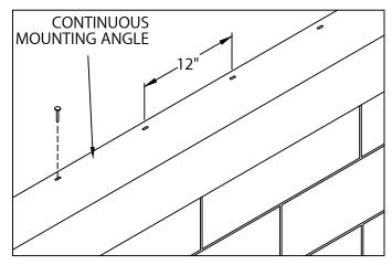
1. OPTIONAL CONTINUOUS MOUNTING ANGLE POSITION CONTINUOUS MOUNTING ANGLE OVER THE ROOF EDGE AND FASTEN 12" O.C. WITH APPROPRIATE FASTENERS FOR SUBSTRATE (SEE NOTE ABOVE). FASTENERS NOT PROVIDED.
