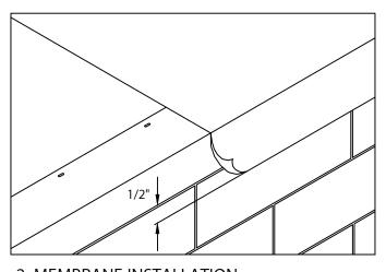
2. MEMBRANE INSTALLATION POSITION MEMBRANE OVER THE ROOF EDGE AND DOWN OUTSIDE FACE OF WALL, COVERING MOUNTING ANGLE AND OR TREATED WOOD NAILER(S) COMPLETELY.
