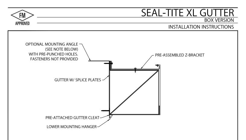
**NOTE:** IF EXTERIOR OF THE BUILDING CONSISTS OF AN INSULATED PANEL, EIFIS, OR OTHER NON-STRUCTURAL MATERIAL, A MOUNTING ANGLE IS REQUIRED WITH THE LOWER MOUNTING HANGER.
