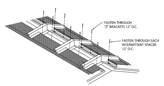
SET RIDGE VENT IN PLACE CENTERED OVER RIDGE OPENING. FASTEN THROUGH PRE-PUNCHED SLOTTED HOLES IN INTERMITTENT SPACERS AT 12" O.C. WITH APPROPRIATE FASTENERS. ALSO FASTEN THROUGH PRE-PUNCHED SLOTTED HOLES IN "Z" BRACKETS 12" O.C.. LAP "Z" BRACKETS 1" ("Z" BRACKETS WILL LAP AND EXPANDED METAL SUPPORT SCREEN WILL BUTT UP TOGETHER).
