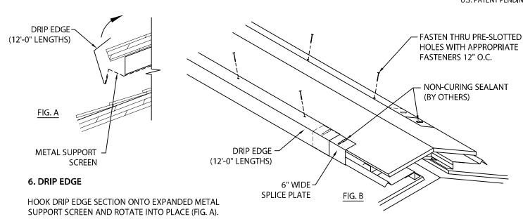
FASTEN THRU SLOTTED HOLES 12" O.C. WITH APPROPRIATE FASTENERS. LOCATE 6" WIDE SPLICE PLATES AT EACH JOINT. APPLY NON-CURING SEALANT (BY OTHERS) TO TOP OF SPLICE PLATE AS SHOWN (FIG B).
