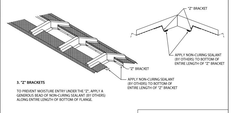
Techni-Flo\* Engineered Roof Ventilation at lasroofing.com
