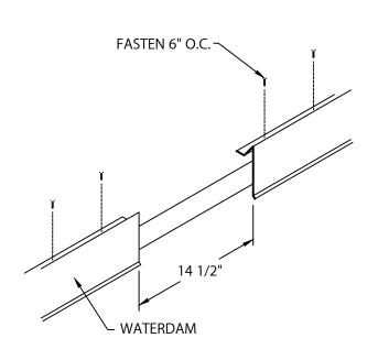
STEP 1 - WATERDAM / ROOFING MEMBRANE DETERMINE LOCATION OF SCUPPER AND SPACE WATERDAM 14 1/2" APART. FASTEN WATERDAM FLANGE 6" O.C. WITH PROVIDED FASTENERS.
