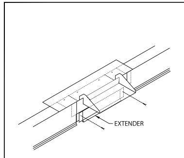
STEP 5- EXTENDER CENTER EXTENDER BELOW SCUPPER AND FASTEN THROUGH PRE-SLOTTED HOLES WITH PROVIDED FASTENERS AS SHOWN.
