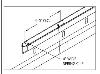
5. INSTALL 12'-0" FASCIA COVER SECTIONS. INSERT ONE SPLICE PLATE AND ONE 4" WIDE SPRING CLIP UNDER FAR END OF FASCIA COVER. PLACE 4" WIDE SPRING CLIPS INTO COVER AT 4'-0" O.C. INSTALL COVER BY PUSHING DOWNWARD UNTIL FASCIA COVER IS ENGAGED TO WATERDAM ALONG ENTIRE LENGTH. CONTINUE TO INSTALL FASCIA COVERS, LEAVING A 3/8" SPACE BETWEEN COVERS. FIELD CUT WHERE NECESSARY USING FINE TOOTH HACKSAW.
