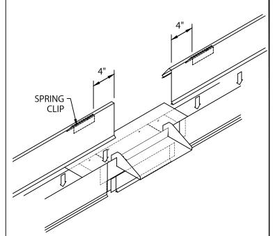
STEP 6- SPRING CLIP / FASCIA COVER PLACE SPRING CLIPS 4" FROM END OF FASCIA COVER. INSTALL COVER BY PUSHING DOWNWARD UNTIL FASCIA COVER IS ENGAGED TO WATERDAM. FASCIA COVER SHOULD FIT TIGHT AGAINST SIDES OF SCUPPER.
