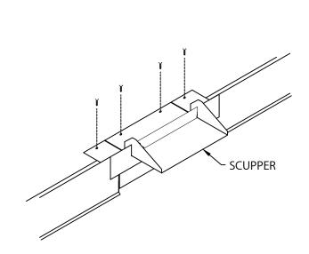
STEP 2- SCUPPER INSTALL SCUPPER WITH PROVIDED FASTENERS. SET SCUPPER FLANGE IN A CONTINUOUS BEAD OF NON-CURING SEALANT.
