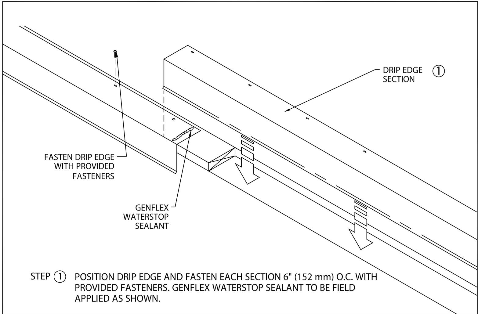
STEP ① POSITION DRIP EDGE AND FASTEN EACH SECTION 6" (152 mm) O.C. WITH PROVIDED FASTENERS. GENFLEX WATERSTOP SEALANT TO BE FIELD APPLIED AS SHOWN.
