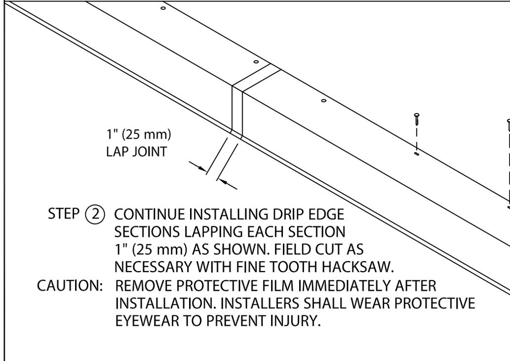
STEP ② CONTINUE INSTALLING DRIP EDGE SECTIONS LAPPING EACH SECTION 1" (25 mm) AS SHOWN. FIELD CUT AS NECESSARY WITH FINE TOOTH HACKSAW.
