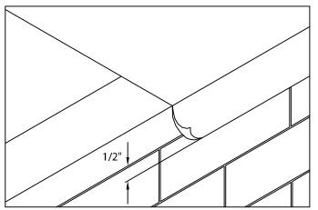
POSITION MEMBRANE OVER THE ROOF EDGE AND DOWN OUTSIDE FACE OF WALL, COVERING TREATED WOOD NAILER(S) COMPLETELY. ALLOW ½" EXCESS MEMBRANE.
