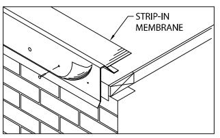
POSITION STRIP-IN MEMBRANE OVER AND DOWN WATERDAM FACE APPROXIMATELY 1" BELOW RAISED FASTENING HOLES (PROVIDED). TAKE CARE TO AVOID BRIDGING OF MEMBRANE. LOCATE AND NAIL MEMBRANE AT 12" O.C. THROUGH ALL RAISED HOLES ON OUTSIDE FACE USING 1 1/4" RING SHANK NAILS PROVIDED.
