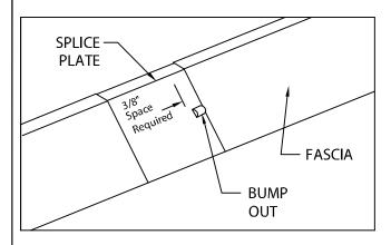
5. INSTALL 12'-0" FASCIA COVER SECTIONS. INSERT ONE SPLICE PLATE UNDER EACH OF THE FASCIA COVERS. INSTALL COVER BY PUSHING DOWNWARD UNTIL FASCIA COVER IS ENGAGED TO WATER DAM ALONG ENTIRE LENGTH. CONTINUE TO INSTALL FASCIA COVERS, FIELD CUTTING WHERE NECESSARY USING FINE TOOTH HACKSAW.
