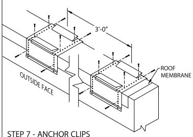
LOCATE OVER ROOFING MEMBRANE AND FASTEN GALVANIZED ANCHOR CLIPS TO WALL AT 3'-0" CENTER WITH PROVIDED FASTENERS AS SHOWN IN DETAIL A
