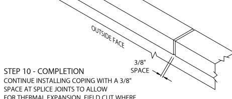
FOR THERMAL EXPANSION. FIELD CUT WHERE NECESSARY USING FINE TOOTH HACKSAW OR SNIPS. NOTE: REMOVE PROTECTIVE FILM IMMEDIATELY.
