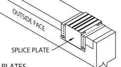
STEP 8 - SPLICE PLATES PLACE SPLICE PLATE ONTO ANCHOR CLIPS AT SPLICE JOINTS, 12'-0" O.C.
