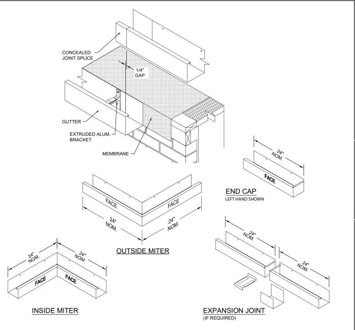
Standard gutter miter leg lengths are 24" Nominal Standard gutter miter angle is 90°
