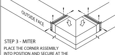
EXPOSED EDGE OF THE ANCHOR CLIPS AS PER DETAIL A. OUTSIDE FACE
