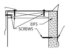
If using an EIFS system, fasten through face w/ fastener of proper length to penetrate through EIFS and attach into structural component
