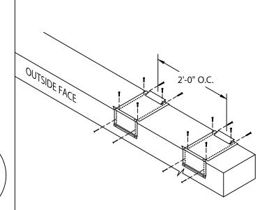
STEP 7 - ANCHOR CLIPS LOCATE OVER MEMBRANE AND FASTEN GALVANIZED ANCHOR CLIPS TO WALL AT 2'-0" ON CENTER WITH PROVIDED FASTENERS AS SHOWN IN DETAIL A.
