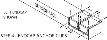
LOCATE AND FASTEN GALVANIZED ANCHOR CLIPS TO WALL WITH PROVIDED FASTENERS FOR SUBSTRATE (SEE DETAIL A). STEP 5 - ENDCAP SPLICE PLATES
