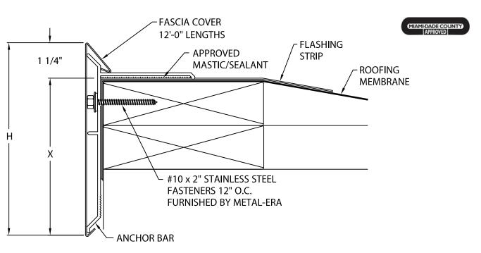
Fascia is to be installed per Specifications and Metal-Era's Installation Instructions Dwg. #11110-1128. for a Built-Up Roof or Modified Roof Systems
