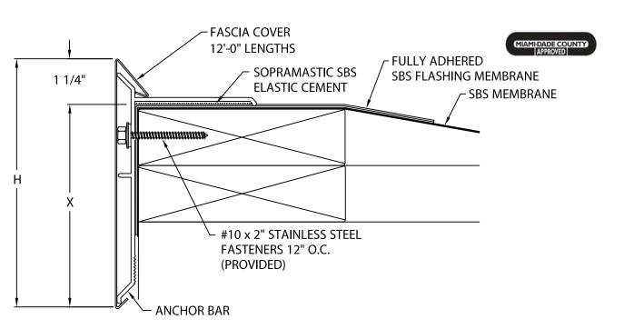
Fascia is to be installed per Specifications and SOPREMA's Installation Instructions Dwg. #33110-13459.
