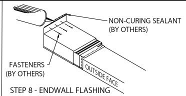
FASTEN TO WALL USING APPROPRIATE FASTENERS (BY OTHERS) AS SHOWN. APPLY NON-CURING SEALANT (BY OTHERS) TO CAULK CUP ATOP 3" FLANGE.
