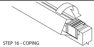
HOOK OUTSIDE FACE OF COPING OVER THE ANCHOR CLIPS AND ROTATE INTO PLACE. ENGAGE REAR LEG ONTO ANCHOR CLIPS BY PRESSING DOWNWARD UNTIL SNAP LOCK OCCURS.
